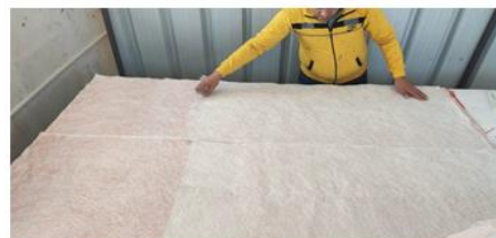
Fig 8. Cutting the fiberglass two layers to fit the mold
