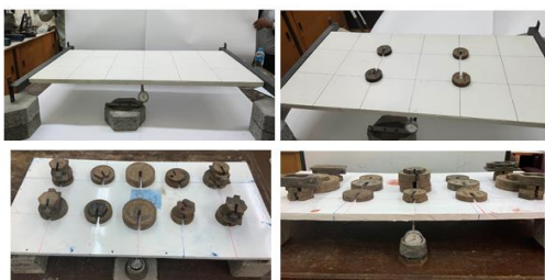
Fig 12. Test setup and bending test for panel
