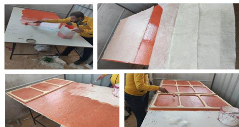
Fig 9. Fabrication of the GFRP wood panel by hand layup procedure
