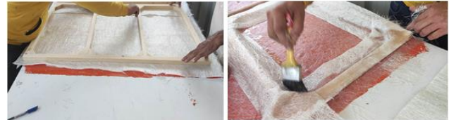
Fig 7. Covering the wooden frame by fiberglass from all directions
